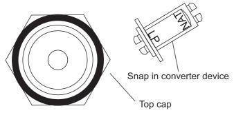
In the base of the brass top is a plastic snap in converter device.
